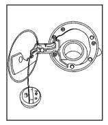
While refueling, hang the fuel cap by the tether using the hook located on the inside of the filler door.
